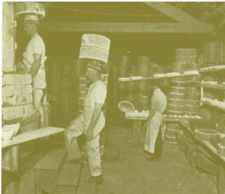
Wares are placed in saggers to protect them from fluctuations in the intense heat of the kiln. Here, workers loading a kiln carry saggers on their heads.
